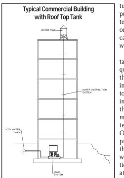
would either turn on to pump more water to the tank or turn off because the tank was full.
