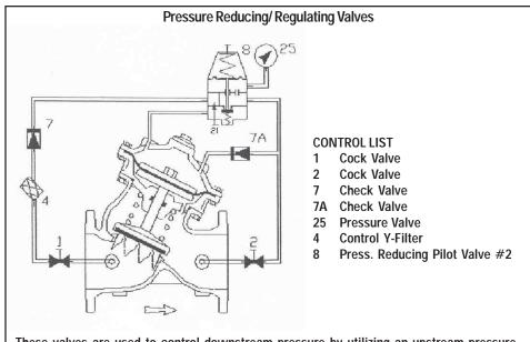
These valves are used to control downstream pressure by utilizing an upstream pressure pilot line feeding a regulating valve. The regulating valve controls pressure supplied to the top of the main valve bonnet. By regulating the pressure on the valve bonnet, the downstream pressure can be regulated. Additional PRVs installed at high energy costs can be added for stability and reponse times.
